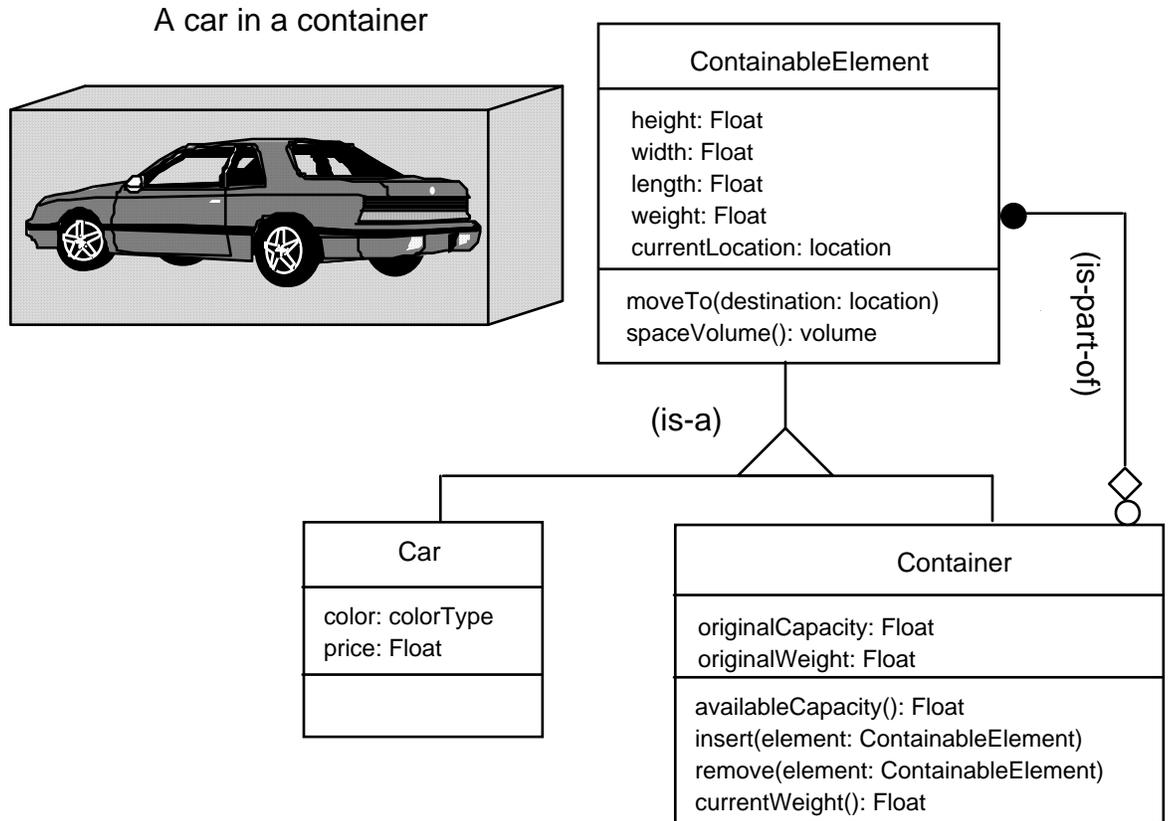
*Figure 7: Object diagram of car and container*
