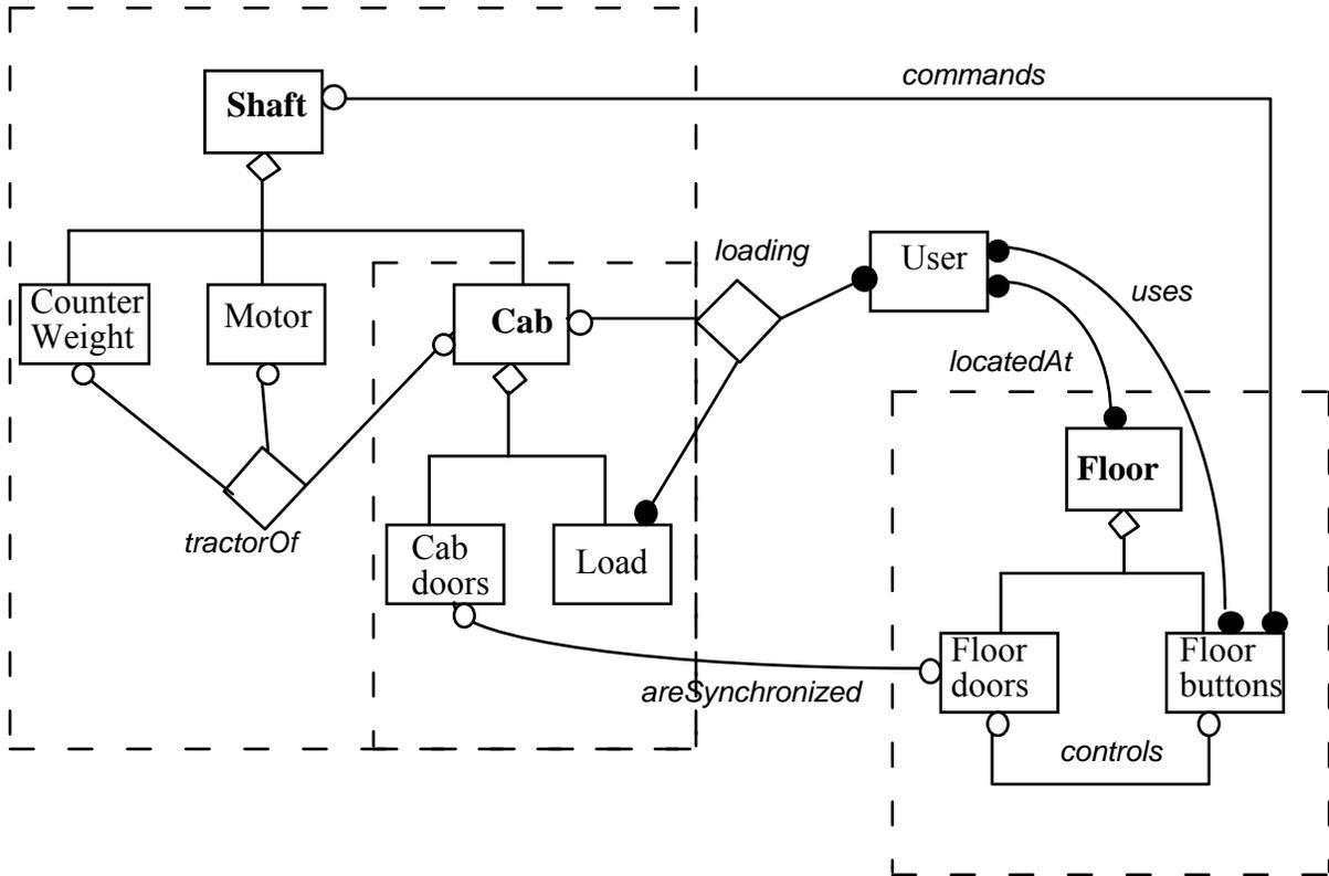
Figure 9: Object model of the lift problem
