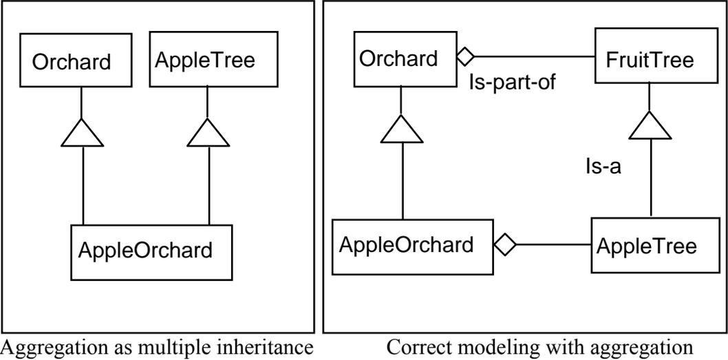
Figure 4: Example of modeling aggregation with multiple inheritance
