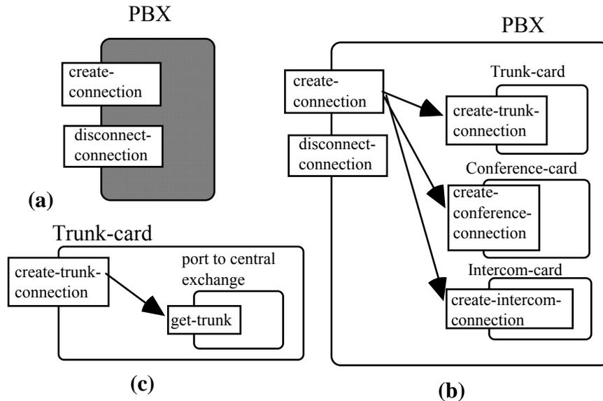
Figure 5: Top-down design example of a PBX
